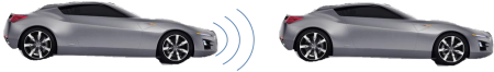
Figure 1: An autonomous car driving behind a leading car uses its distance and velocity sensors to make a braking decision.
